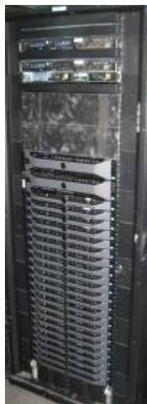
Avalanche is the newest cluster at FEUP, being purchased at the start of 2013. It has 29 nodes, each with 16 cores and between 64GB and 128GB of RAM. Each node is connected via a 40Gbps InfiniBand network. There is 10TB of central storage, with each node having 500GB of local storage. The clusters run version 7 of the [Scientific Linux](#) operating system (a distribution based on Red Hat Enterprise Linux 7) from CERN and Fermilab.
